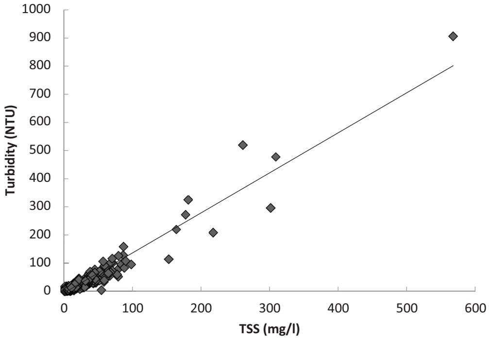
**Figure 31: Scatterplot to illustrate the linear relationship between turbidity and Total Suspended Solids (TSS).**
