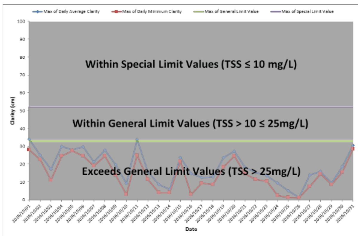
**Figure 34: Summary data for Howick WWTW compliance with various DWS limits, using a calibrated water clarity tube.**
