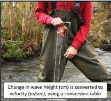
Change in wave height (cm) is converted to velocity (m/sec), using a conversion table
