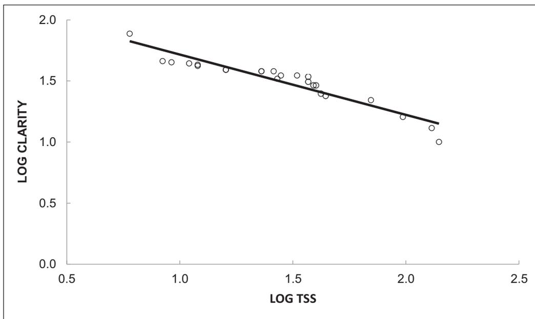
**Figure 33: Scatterplot illustrating the relationship between Log10Clarity (LOG CLARITY) and Log10Total Suspended Solids (LOG TSS). The solid line represents the trend in the data set.**
