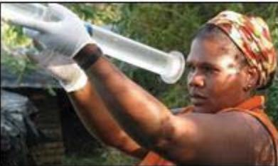
In 2013 the water clarity tube was calibrated to measure water clarity relative to discharge limits of total suspended solids set by government standards.
