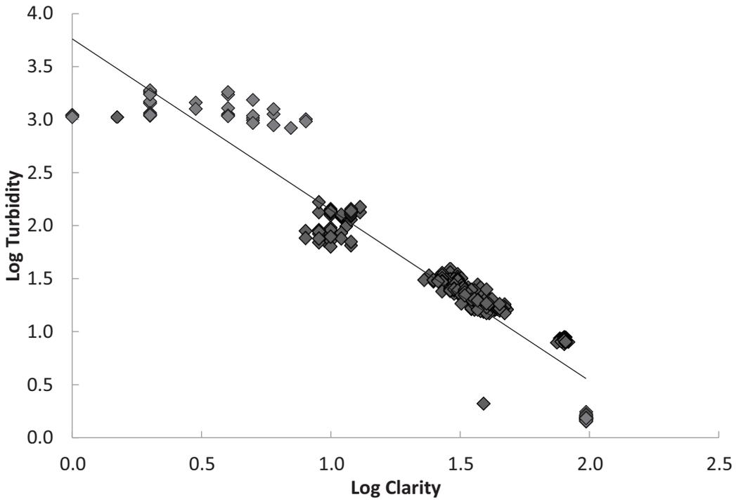
**Figure 30: Scatterplot to illustrate the linear relationship between log-transformed values of clarity and log-transformed values of turbidity for *in situ* and *ex situ* samples.**
