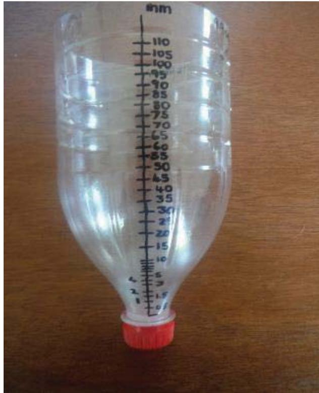
**Figure 40: Recycled Coca-Cola bottle CS rain gauge**
