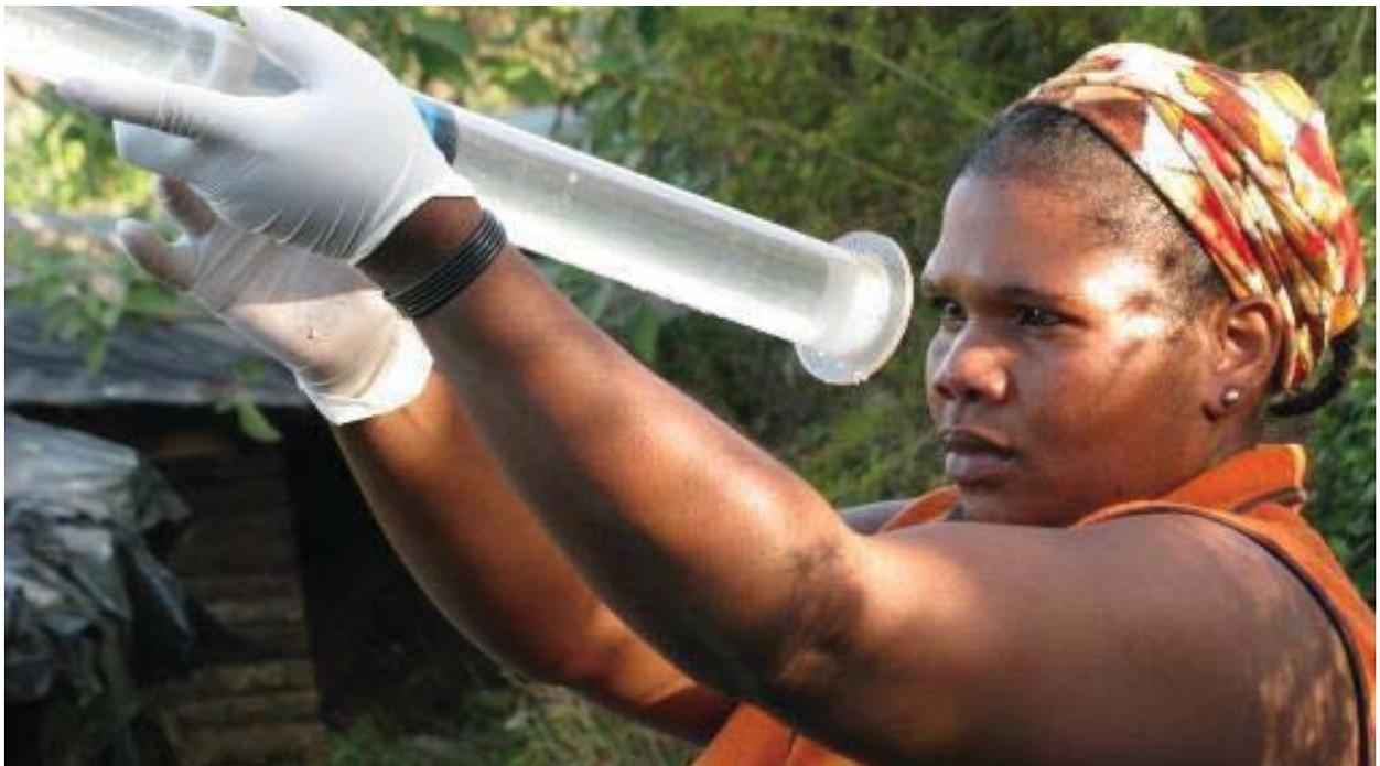
**Figure 50: Few people realise that nutrient loading is a massive risk to most rivers and streams in South Africa. Here Zongile Ngubane measures the water clarity of the Wastewater treatment Works (WWTW) outflow pipe in Shiyabazali informal settlement. Clarity measurements are converted to represent total suspended solids, which include nutrients (photo courtesy of Andrea Kolbe).**
