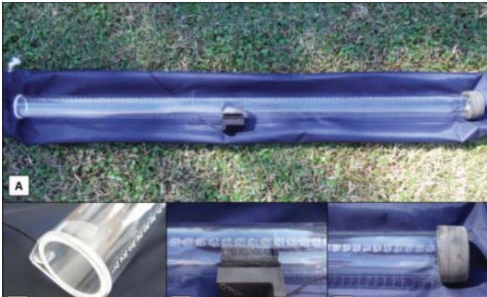
**Figure 27: Components of a water clarity tube. A: The full length of the tube, with the protective cover; B: Clear base for viewing the disk; C: Magnets for moving disk; D: Black stopper-cap for sealing the tube**
