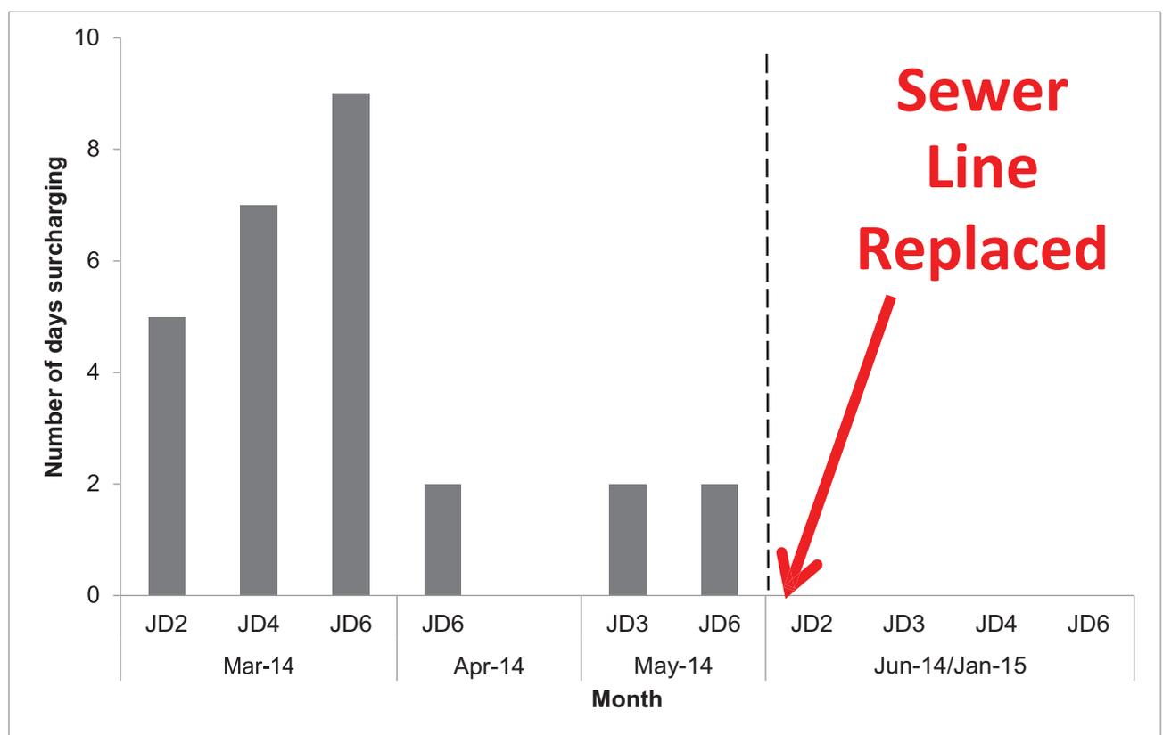
**Figure 59: Sewer line monitoring data from Mpophomeni showing the number of days per month sewer lines surcharged (as monitored by EnviroChamp Jabulani Dladla) and results after the sewer line was replaced.**
