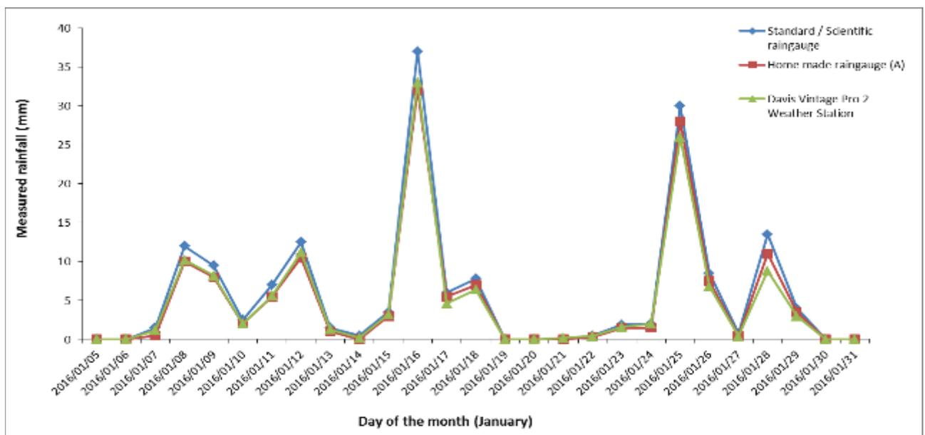
**Figure 41: Graph showing the data collected from a CS rain gauge, a standard/scientific rain gauge and a Davis Vintage Pro 2 Weather Station over one month**
