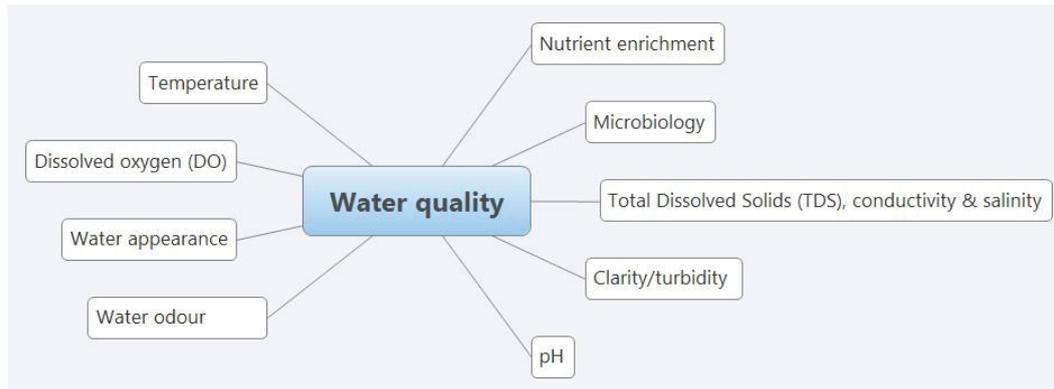
**Figure 5. Various water quality parameters identified for measuring in streams and rivers.**
